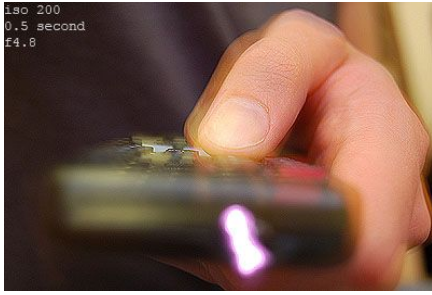
Nikon D50. ISO 200, 1/2 second, f4.8. This camera is very sensitive to IR light :)
